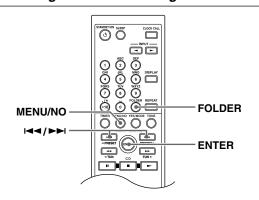
With Navigation mode, you can select MP3 files by navigating through the folder hierarchy. This mode can only be used while playback is stopped.
